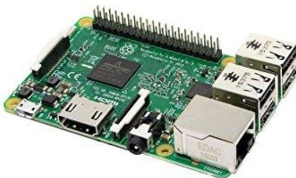
Figura 87. Raspberry Pi 3 Modelo B.
