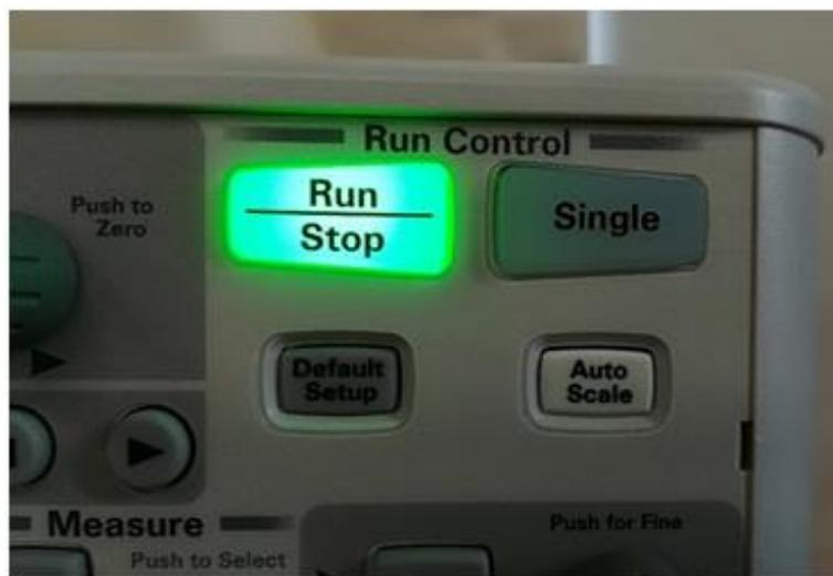
Figura 53. Panel RUN CONTROL, tecla Run/Stop.
