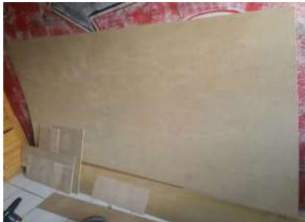
**Figura 30.** Tabla Triplex de 4mm
