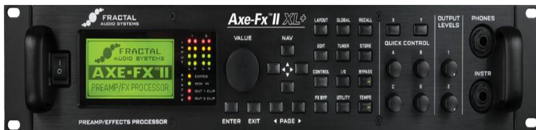
Figura 44. Rack amp modeler, Fractal audio Axe Fx II Tomado de Fractalaudio.com, 2016
