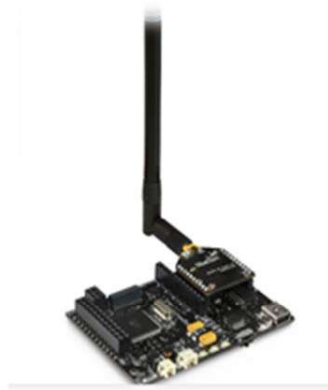
Figura 10 Wasp mote with LoRa Radio + 4dBi antenna
