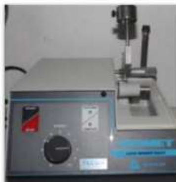
Figura 14. Máquina de corte (Isomet Low speed Saw, Buehler, Lake Bluff, Illinois USA)
