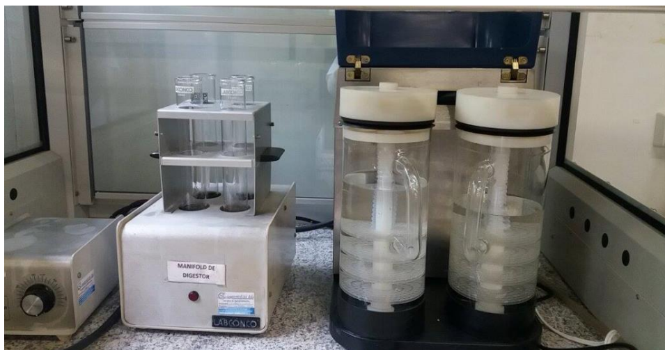
Figura 11. Manifold de Digestor
