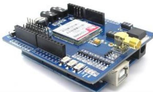
IComsat is a GSM/GPRS shield for Arduino and based on the SIM900 Quad-band GSM/GPRS module. It is controlled via AT commands (GSM 07.07, 07.05 and SIMCOM enhanced AT Commands), and fully compatible with Arduino / Iteduino and Mega.
