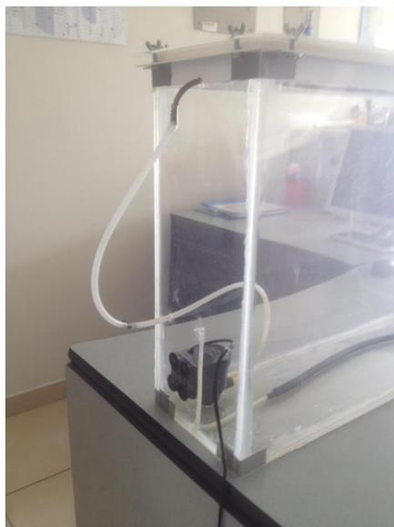
Figura 6. Detalle biorreactor, bomba sumergible.
