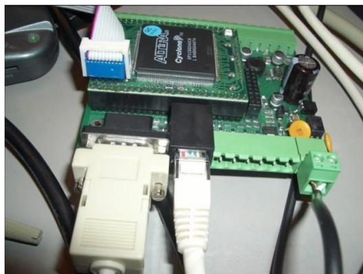
Figura 32. Placa Java Optimized Processor
