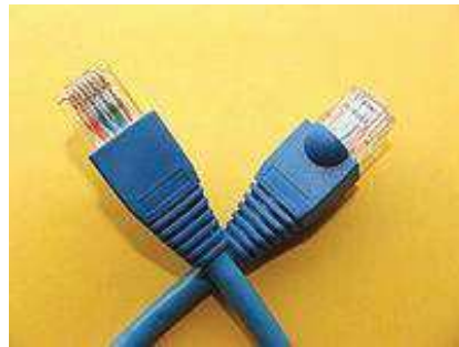
Fig.2 Cable utp Rj-45
