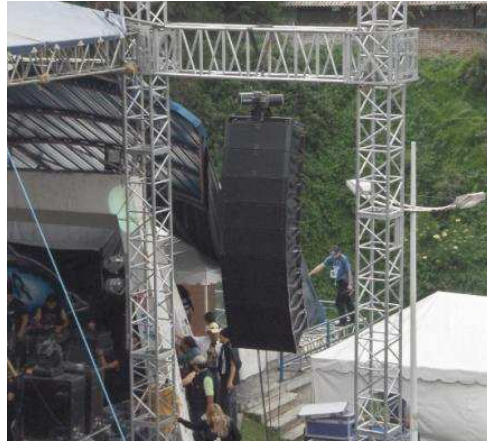
Figura 4.21. Line array Electro Voice dvx 127.
