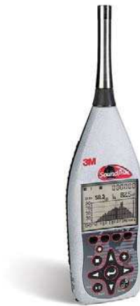
Figura 2.4. Sonómetro QUEST TECHNOLOGIES SoundPRO SE/DL Series
