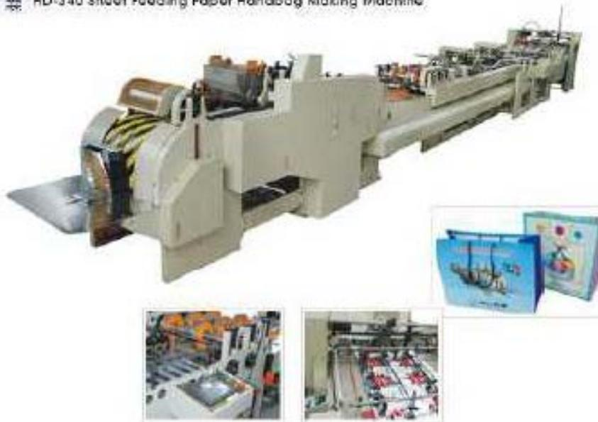
This machine produces square bottom bags from paper sheet or printed paper sheet. The fed materials can be either single printed sheet paper or laminated paper as per end-user's preference. This machine features a continuous function of automatic paper feeding, gluing, creasing, bottom-folding, bottom-gluing and bag forming at a stroke.
