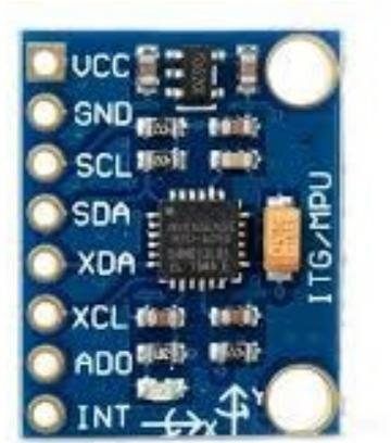
Figura 4. Sensores (IMU) MPU6050
