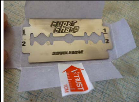
Remark 1: poor printing for the marking on product
