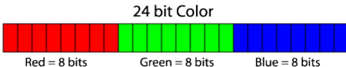
Figura 3 Profundidad de 8 bits de un píxel digital con color en 24 bits. Tomado de: https://www.researchgate.net/figure/Color-Information-Pixel-uses-a-total-of-24-bits-8-bits-for-red-8-bits-for-green-and-8_fig1_333570725
