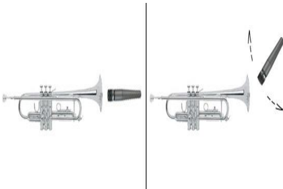
Figura 25. Ubicación On axis y Off axis . Bagley, K. Tomado de: How to Record Horn, Brass and Saxophone Players in the Studio.
