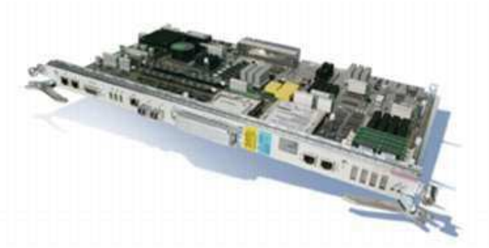
Figura 32. Cisco CRS 8-Slot Line-Card Chassis Route Processor Tomado de (Cisco, 2015)
