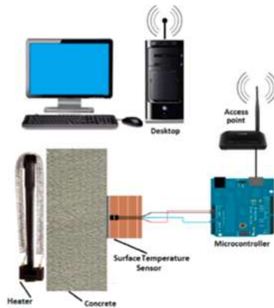
Figure 9. Electrical diagram of the test bench used in the validation tests.
