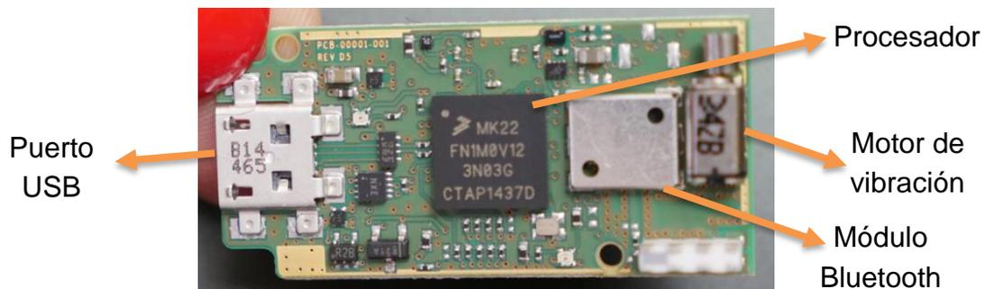
Figura 19. Placa principal del MYO Armband.
