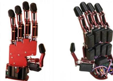
*Figura 5.* AR10 Humanoid Robot Hand.
