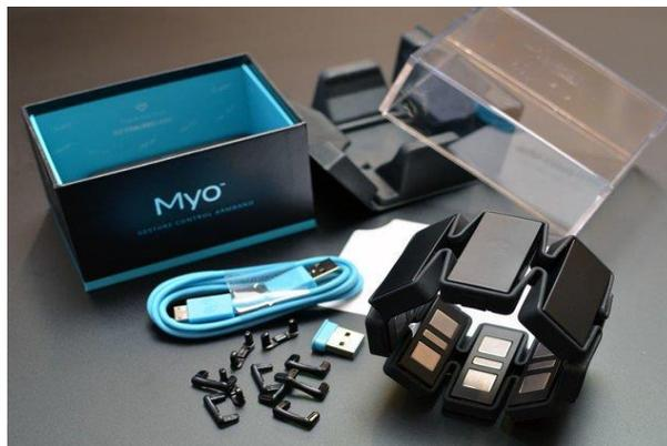
*Figura 15.* MYO Gesture Control Armband.
