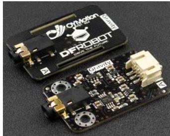
*Figura 14.* Gravity: Analog EMG Sensor by OYMotion.
