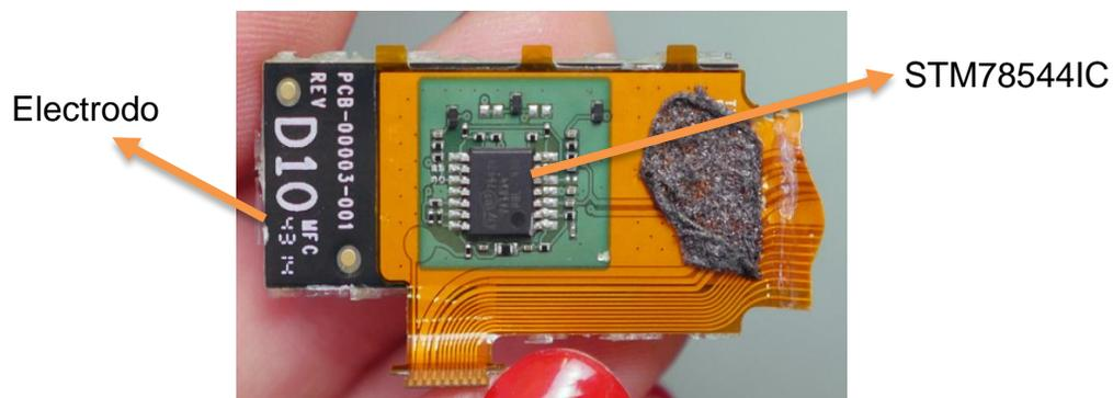
Figura 20. Placa principal del MYO Armband.
