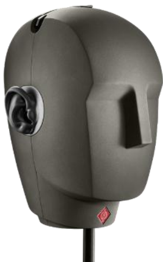
Figura 6. Dummy Head Neumann KU100.
