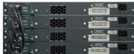
Figure 2. Cisco FlexStack Switch Stack
