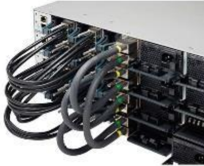
Figure 2. StackWise 480 and StackPower Connectors
