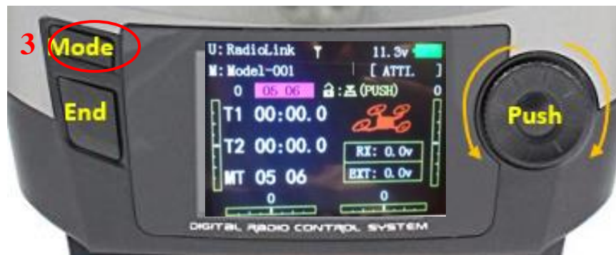
Figura 86. Interfaz Principal del Control AT9
