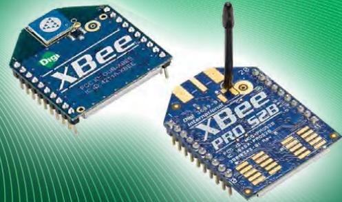
Embedded RF modules provide low-cost, low-power wireless connectivity using the ZigBee PRO Feature Set.
