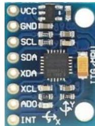
Figura 1. sensor MPU-60-50
