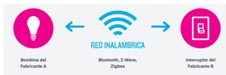
Figura 1. Arquitectura Device to Device .
