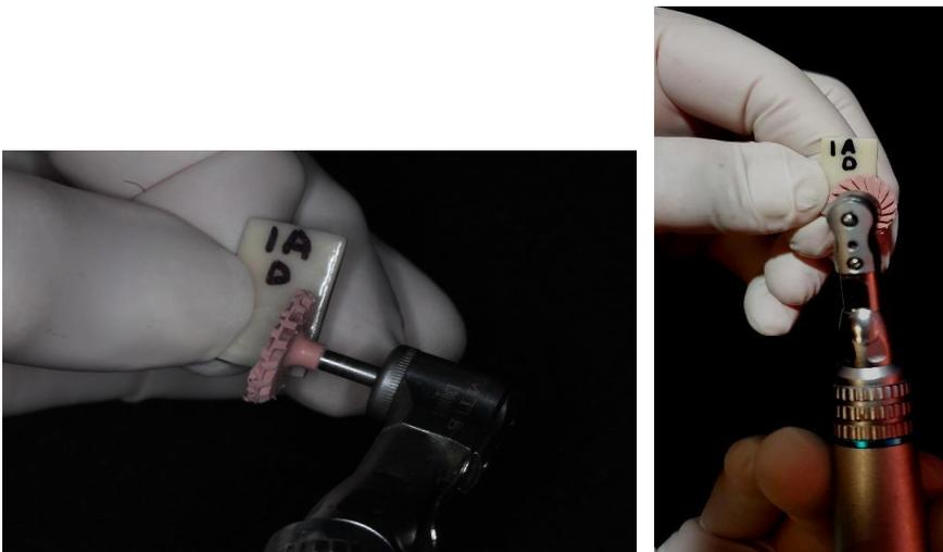
Figura 7: Pulidor de cerámica de diamante: segundo paso (Intra- oral Dialite HP Porcelain Adjustment Polishing kit k0193, Diatech, USA). (Intra- oral Dialite HP Zirconian Adjustment Polishing kit Diatech, USA).
