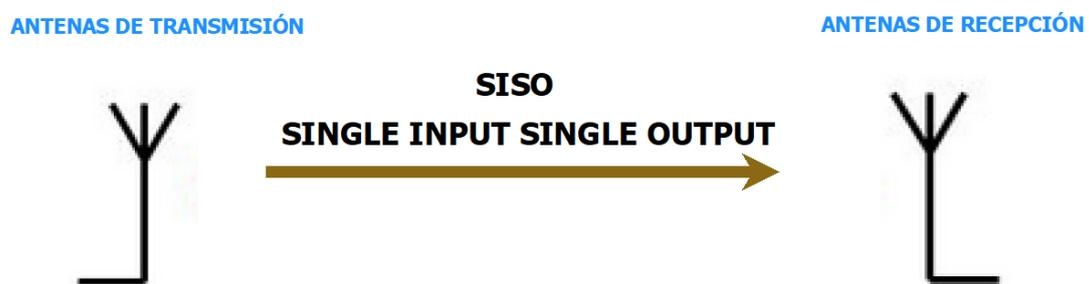
Figura 6. Arquitectura SISO (*Single Input Single Output*)
