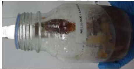
MUESTRA CONTAMINADA CON MUD FLUSH A LAS TRES HORAS GENERA UN GEL VISCOSO
